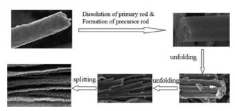
A single-layer polycrystalline anatase  ${\rm TiO_2}$  nanosheet with a porous structure was synthesized through a simple solvothermal synthetic method, followed by calcination.
